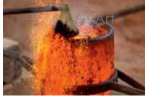
Clearing oxide from the molten bronze
